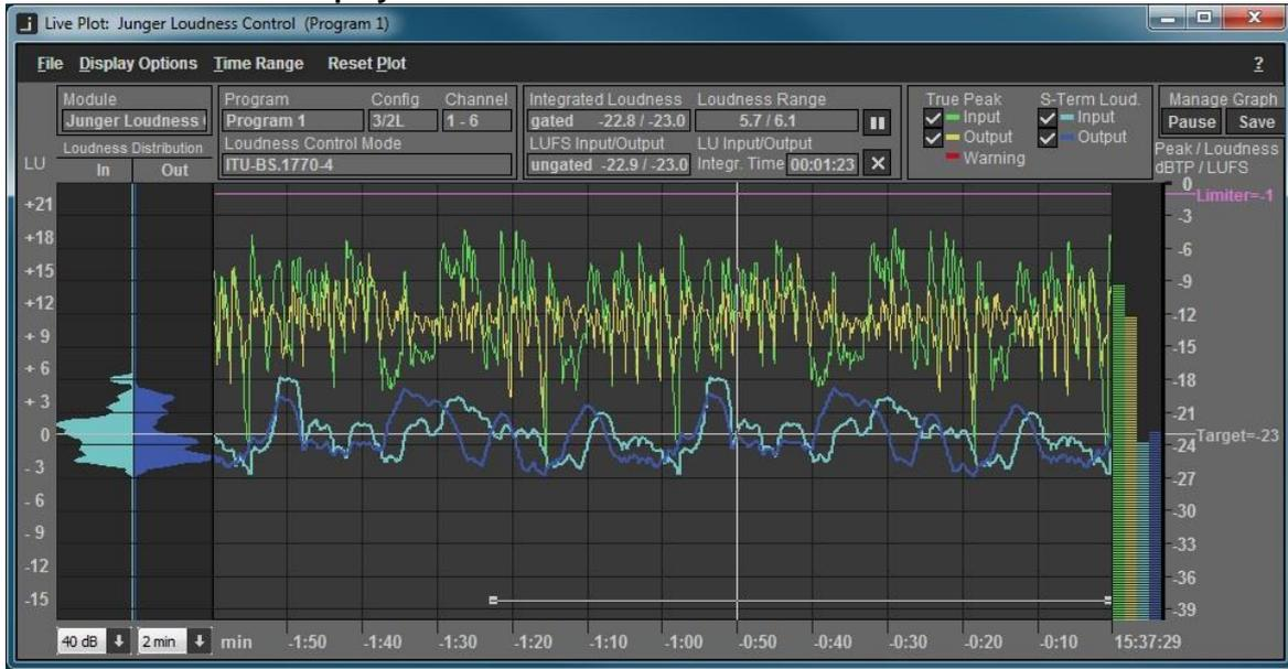
As explained in the previous paragraphs, the values of an integrated loudness measurement will be displayed in the upper area of the plot. In the bottom of the plot you see a horizontal line that represents the selected time frame for the measurement. If you select multiple time frames or if you pause and continue the integrated measurement manually, multiple horizontal lines will be displayed to show the areas which contribute to the overall result.
