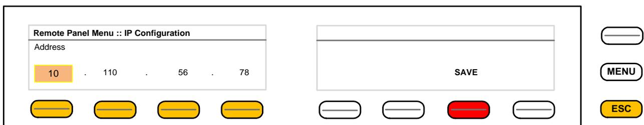
You must press one of the respective **<F-Keys>** and that field will be highlighted as well as the Rotary Encoder. Now you can change the value by turning the knob. When the setting of all fields is finished, you must press **<SAVE>**. The display will return to the initial **"Remote panel Menu"** page 1/3.
